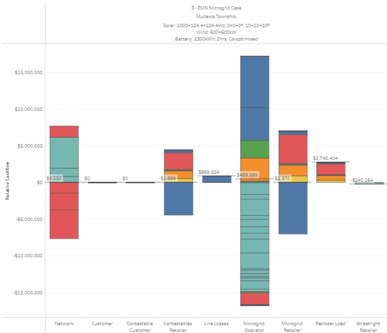
Figure 7-8: Relative cashflow results (relative to current operation today) for RGS+NCS (upper) and EMN (lower) Microgrid Models based on asset sizing of 1000kW Solar, 1200kW Wind & 2300kWh battery
