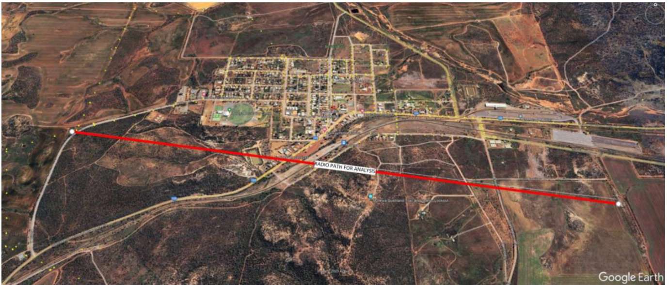
Figure 10-5: Radio path analysed for communications reliability (from Jarrah Solutions FEED Report, Appendix F)
