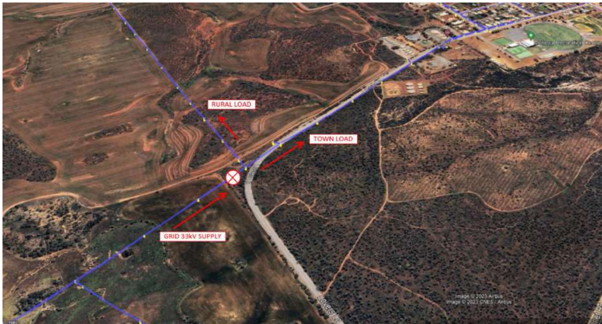
Figure 1: New recloser (crossed red circle) to be installed by Western Power.
