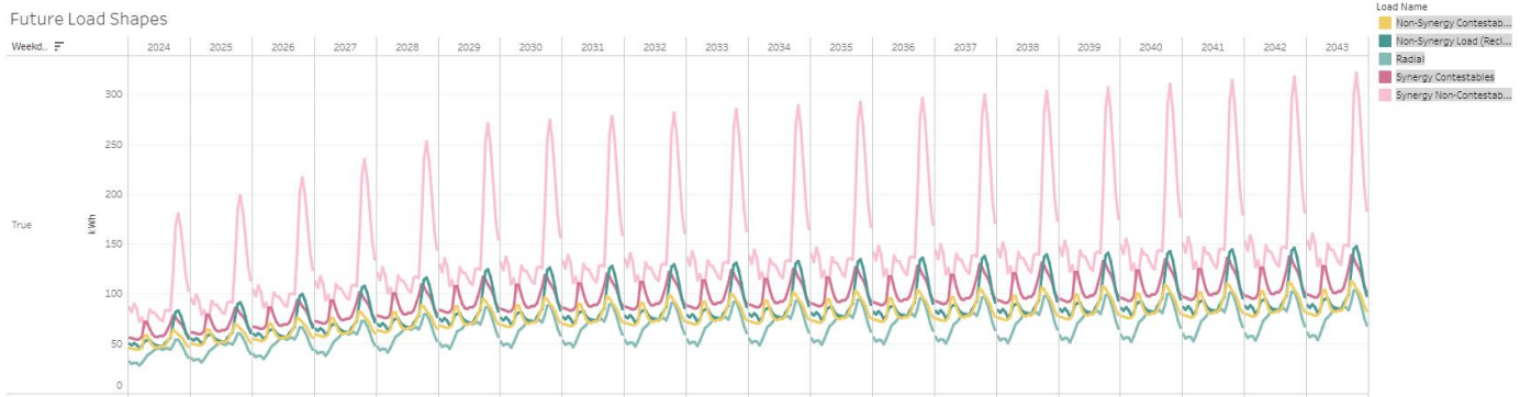
Figure 8-6: GridCog input representing increase in load by 10% per year over 5 years, then reducing to 2% per year for remaining years
