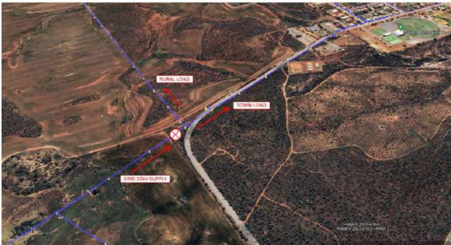
Figure 3-3: New recloser (crossed red circle) to be installed by Western Power
